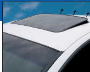
Sunroof panel vents for interior comfort, or opens fully for added exposure.
